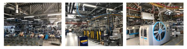
The newspaper printing plant of NZZ Media Services AG in St. Gallen-Winkeln is now equipped with Ferag mailroom technology. Two MultiSertDrum are the centre of attention. The bundles are formed by six MultiStack compensating stackers.
